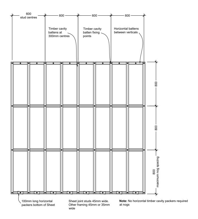
**Note:** Horizontal packers must be set to a fall of 5° minimum where shown
